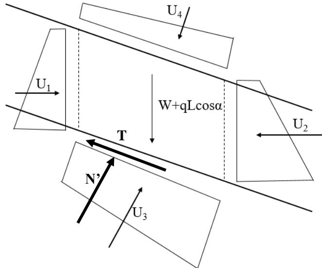
2. For a flow parallel to the slope, compute  $F$  at  $z = H$  using two alternative approaches to account for the water flow: (i) total weight of the soil and pore water pressure distributions along the sides of the soil slice, (ii) buoyant weight of the soil and seepage force.
