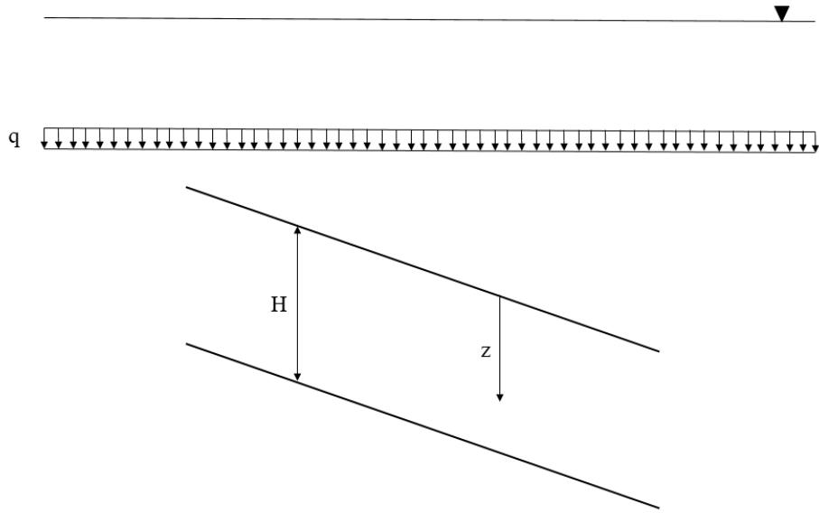
The constant external vertical stress acting on the extrados of the slope can be included in the analysis considering the contribution of an equivalent vertical force per unit of width,  $P=q L \cos\alpha$  acting on the considered slice of soil:
